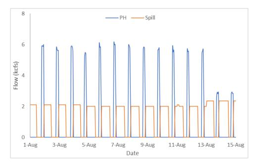
Figure 23. Hourly Flows PWR vs. Spill (Lookout Dam Tailrace)
