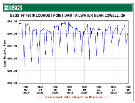
Figure 20. Gauge Height (feet); below Lookout Dam.
